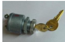
Universal OFF/ON(IGN) 2 Position Key Switch (For Battery Ignition) (2 Screw Terminals) Mounting Stem 3/4"-20 Thread
